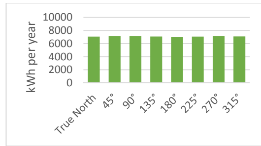
Figure 15 Comparison of the Bar Orientation of Type A Terrace House Total Energy Use in 45° step stages from True North, 0, with 10% WWR on both ends of the terrace house
